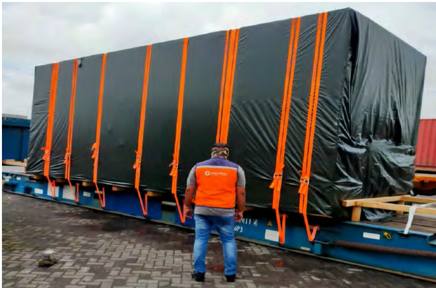
Proper Lashing & choking before exports from India
